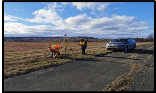
Figure 4- Courtney Roddick, CLS, and André Bédard setting up a GPS receiver over NB control monument 5510 (ME/NB)
