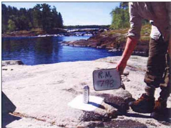
A Reference Mark after it has been cleaned and painted – Minnesota / Ontario
