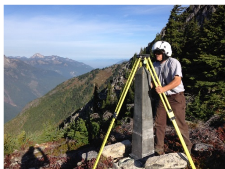
Figure 5 – Setting up a GPS receiver over Monument 56 (British Columbia/Washington)
