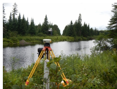
Figure 2 – State-of-the-art GPS receivers set over Monuments 304 and 305 (Quebec/Maine)
