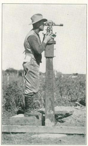
OBSERVING FROM A BOUNDARY MONUMENT. NOTE SPECIAL DEVICE FOR MOUNTING THE THEODOLITE
